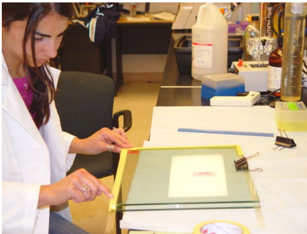
Supplemental Figure 8: Again, proper taping on all sides of the glass plates cannot be emphasized enough as liquid acrylamide leakage may occur from improper taping. One should be certain that the tape is tightly adhered on all sides and especially the bottom.
