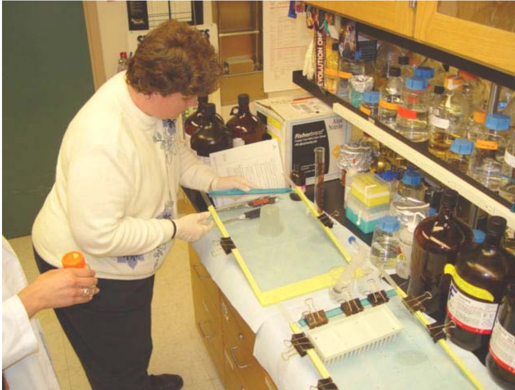
Supplemental Figure 11: Once the gel has been properly poured, thoroughly check for bubbles and remove any bubbles with a bubble buster (a thin wire apparatus designed to assist in bubble removal). Then carefully place a one-well comb between the plates at the top.
