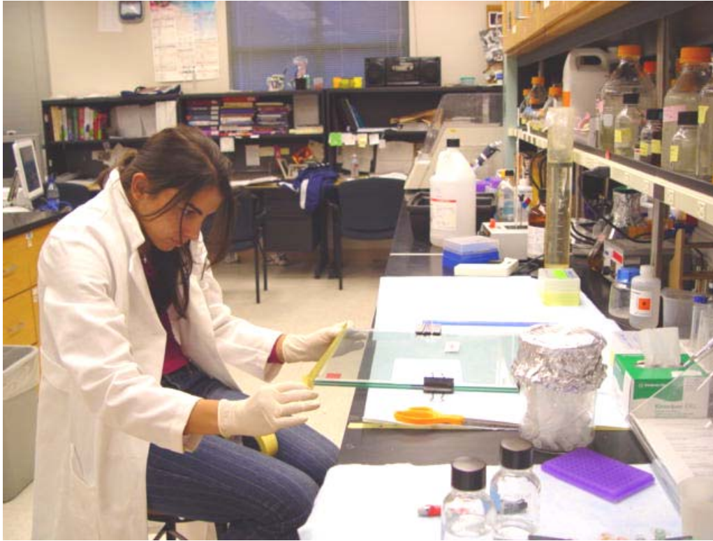
Supplemental Figure 7: It is recommended to cut the tape the length of the plates and utilize the tape so half will be adhered to the top plate while the other half will be adhered to the bottom plate, as illustrated in above figure. Be sure that while taping, the other sides of the plates remain tightly clamped.
