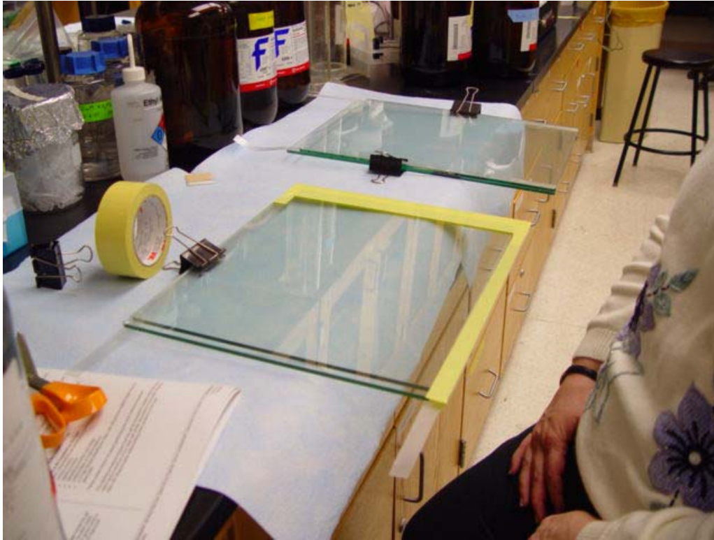
Supplemental Figure 6: Carefully remove the clamps from one side and thoroughly tape with highly adhesive electrophoresis tape. It is important to verify that the tape is securely adhered to the glass, otherwise it will leak when the gel is poured between the plates.
